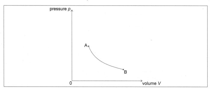
Process AB is an isothermal change, as shown on the pressure volume (pV) diagram, in which the gas expands to three times its initial volume.
