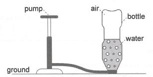
The air-water mixture is called the propellant.
