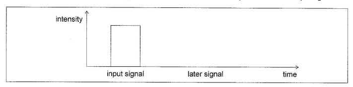
Sketch, on the axes, the variation of signal intensity with time after the signal has travelled a long distance along the fibre.
