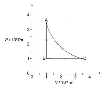
The heat pump transfers thermal energy to the interior of a building during processes  $C \rightarrow A$  and  $A \rightarrow B$  and absorbs thermal energy from the environment during process  $B \rightarrow C$ . The working substance is an ideal gas.
