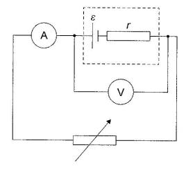
The current I and the terminal potential difference V are measured.
