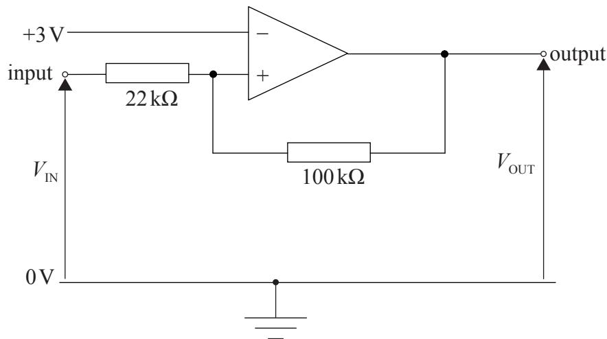
The output of this Schmitt trigger is positive saturation ( $+13\text{ V}$ ) or negative saturation ( $-13\text{ V}$ ).
