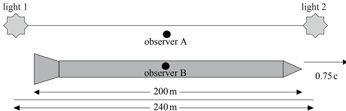
According to observer A, at the instant when observer B passes observer A, the two sources of light emit a flash. Observer A sees the two flashes simultaneously. Discuss whether or not observer B sees the two flashes simultaneously. [4]
