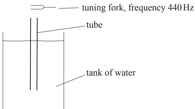
A tube that is open at both ends is placed vertically in a tank of water, until the top of the tube is just at the surface of the water. A tuning fork of frequency 440 Hz is sounded above the tube. The tube is slowly raised out of the water until the loudness of the sound reaches a maximum for the first time, due to the formation of a standing wave.
