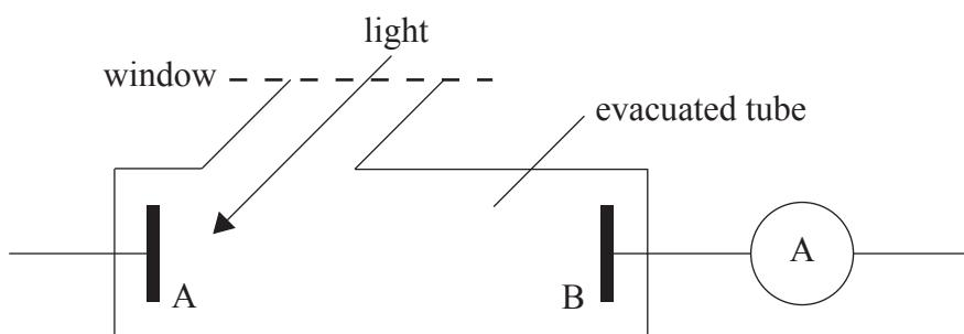
When the frequency of the light is reduced to a certain value, the current measured by the ammeter becomes zero. Explain how Einstein's photoelectric theory accounts for this observation.
