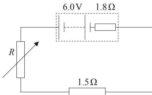
Estimate the resistance  $R$  of the variable resistor that will limit the current to  $0.82\text{ A}$ .
