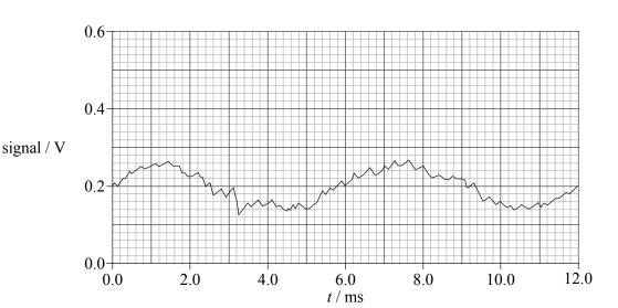
waveform: lower mean signal/power/voltage; smaller amplitude;
